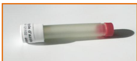
Photo 1 : Tube passif NO 2
