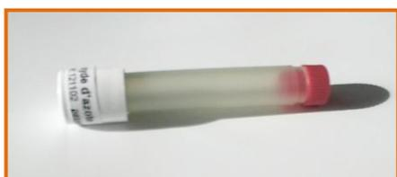
*Photo 1 : Tube passif NO<sub>2</sub>*
